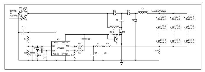
This power factor corrected circuit provides a constant average current output to power LED lamps.
